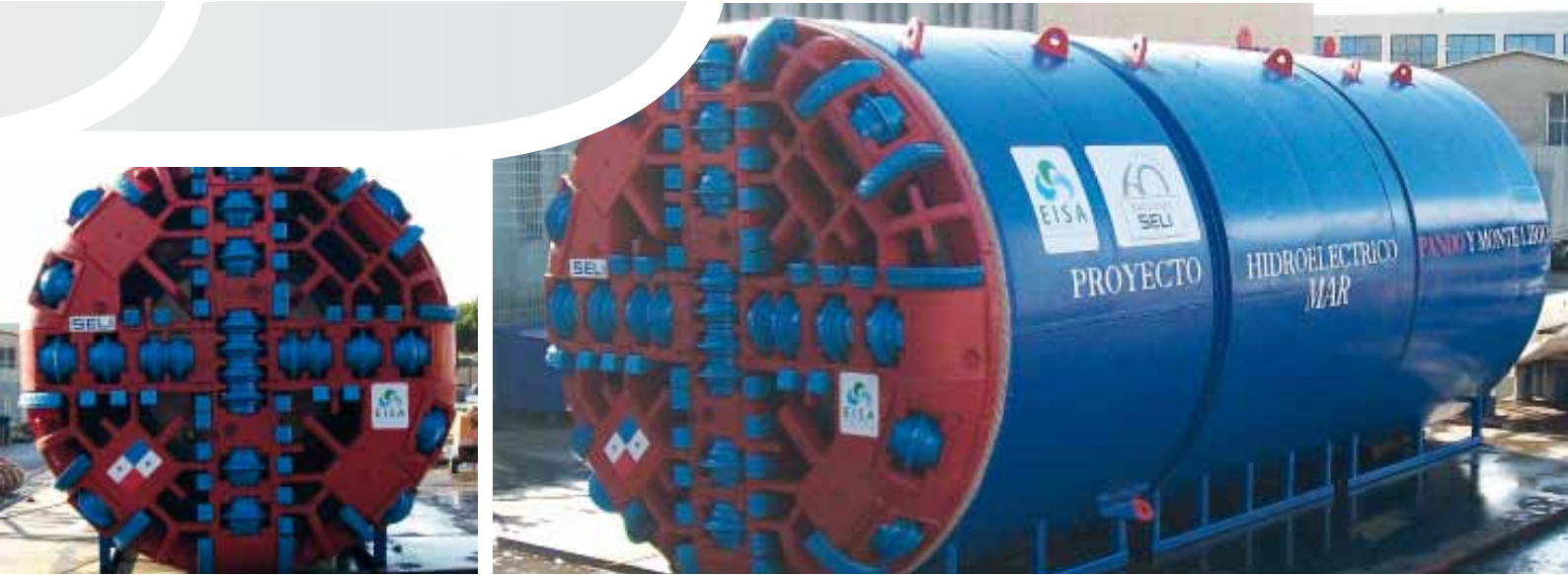
SELI - TBM for the construction of the hydroelectric plant of Pando, Panama
